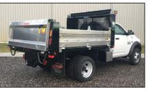
**HYBRID** Steel Body with Aluminum Fold Down Sides & Tailgate
